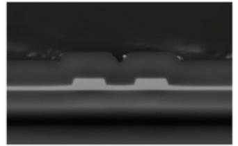
Cross section of an evanescent beamsplitter
