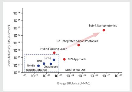
**High performance:** Photonics can run at few tens of GHz bandwidth compared to few GHz in digital electronics, giving more operations performed per second.
