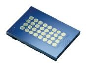
At the heart of this innovation is Q.ANT's proprietary Thin Film Lithium Niobate on Insulator PIC, which offers precise light control at the chip level.
